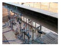
Test in progress: Instrumentation is installed throughout the barrette section and length
